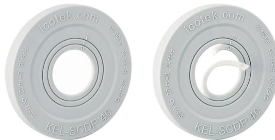
The single membrane rings are peeled off according to the diameter of the routed cable/hose. For this purpose, only a small hole between the rings needs to be pierced. Then the corresponding ring can be removed.
