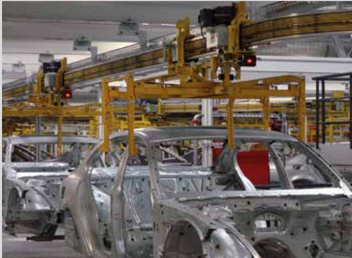
Monorail system with car bodies in the automotive industry
