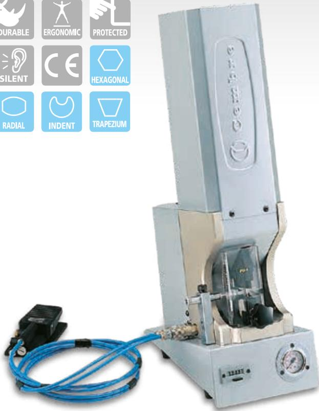
Pneumo-hydraulic, production bench press, controlled by a foot operated pedal, provides a consistent and reliable crimped connection. Extensive range of interchangeable dies available for crimping a wide variety of connectors.
