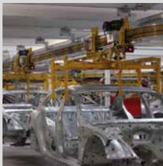
Monorail system with car bodies in the automotive industry
