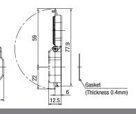
· Panel thickness when CW97-D1X1/D1X2 is mounted: 1.5 to 5 mm
