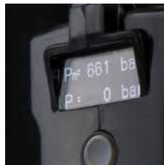
OLED multifunctional display with touch button
