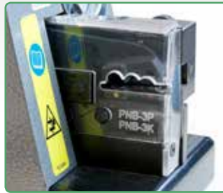
PNB-3P detail of the crimping zone.
