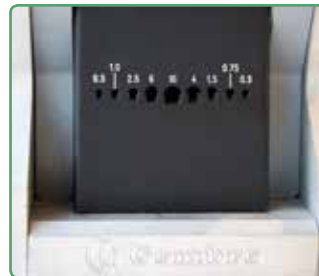
PNB-4KE detail of the crimping zone.
