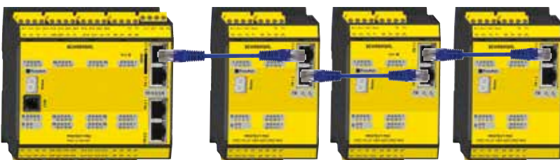
Decentral structure: Expandable with the remote I/O module
