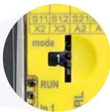
Function setting via rotary knob mode
