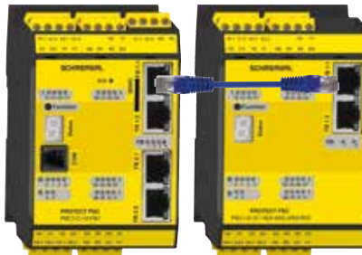
Decentral structure: Expandable with the remote I/O module
