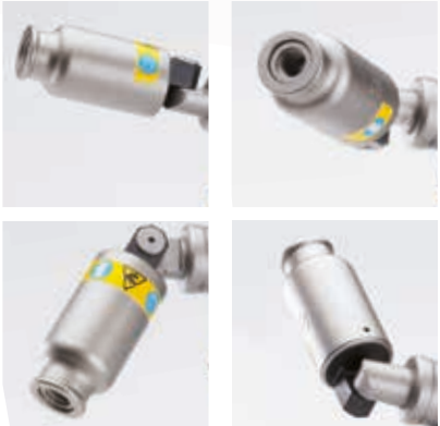
Universal joint allows punching head to pivot 180deg over a full 360deg rotation.
