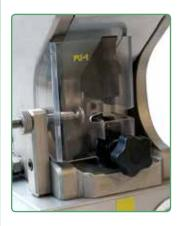
PNB-1 detail of the crimping zone with PU-1 guard.
