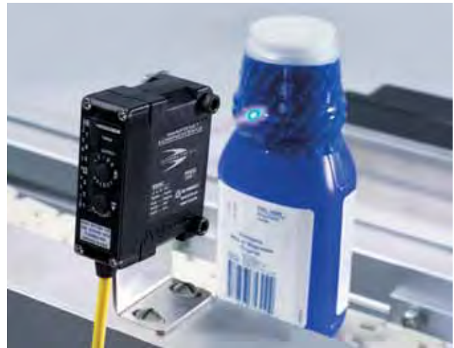
Verification of seals
