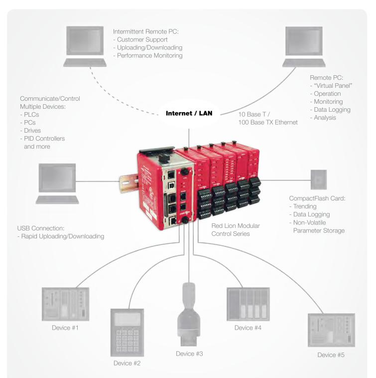
Communicate with up to five different types of serial devices simultaneously. Access, monitor and control these devices from across your network or around the globe.
